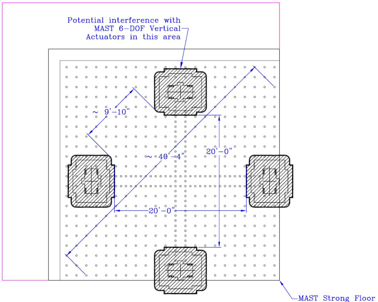
Figure 7. Strong floor interference and working space
