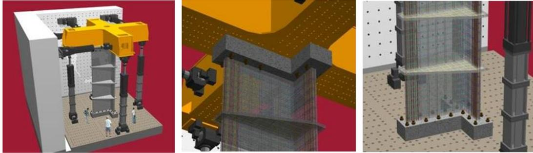
Figure 5. Schematic of 4-story T-wall test specimen
