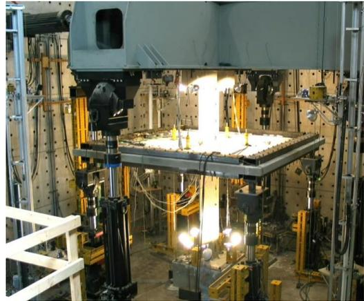
*Figure 4. Slab-Column Subassembly*
