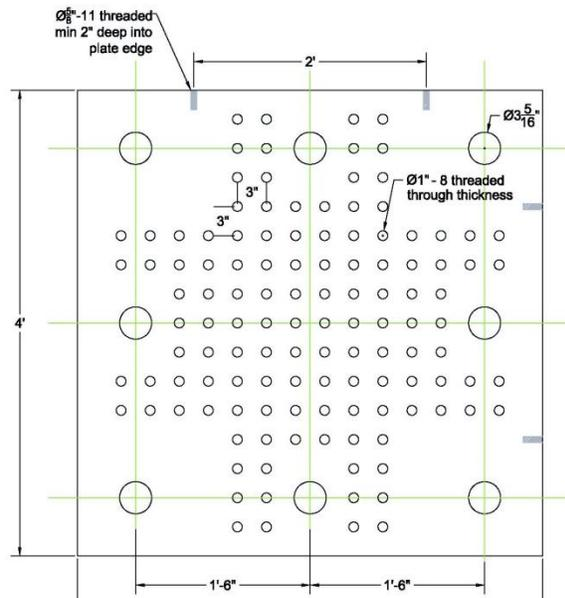
Figure 10. Strong floor/Strong Wall attachment plates
