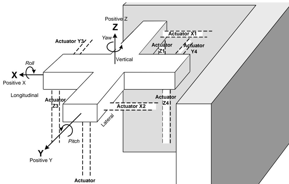
Figure 1. Isometric of crosshead positioned in strong walls
